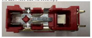
5. Rotate the red fuse holder 180° from its original position, and reinsert it into its housing. For 100/115V operation the voltage displayed on top should be 115.
