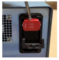
4. To convert from 220/240V to 100/115V, replace the two 1.6 Amp fuses with 3 Amp slow blow fuses. See the picture above for 230V proper fuse position.
